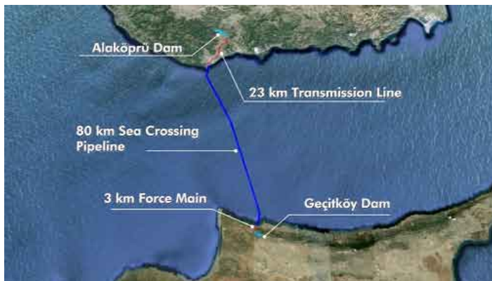
75 million m 3 /year water will be transferred from Turkey to TRNC via a submarine pipeline
