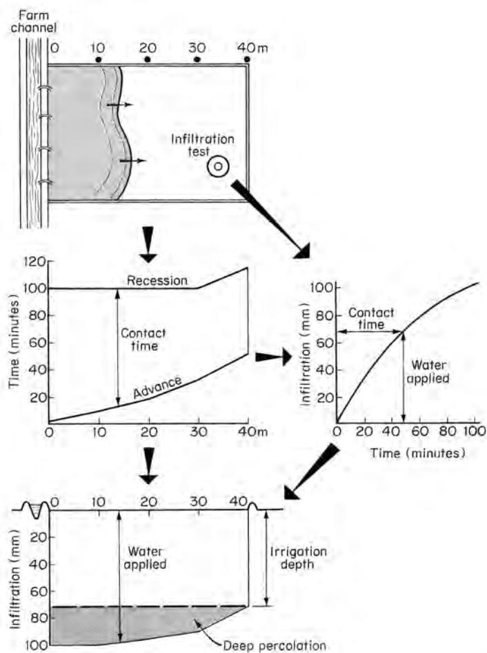
Figure 23 Typical results from a basin irrigation evaluation [55]
