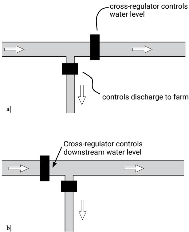
Figure 10 a) Upstream and b) downstream control
