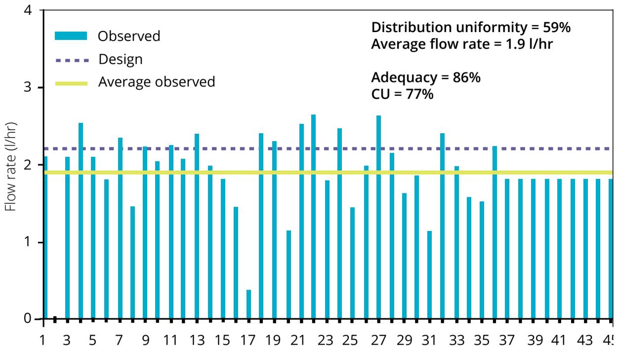
Figure 29 Emitter flow rates measured along a drip line which was two years old.
